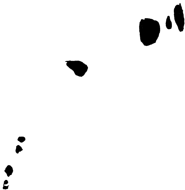
Fig. 6. Two-dimensional TLC separation of fatty acid methyl esters derived from human serum triglycerides. The silica gel-silver nitrate method of deVries (6) was used; the solvent systems were (vertical) ethyl acetate-benzene (88:12) and (horizontal) benzene. The presence of one or more trans -monene compounds is clearly evident in the upper right hand section of the plate.
